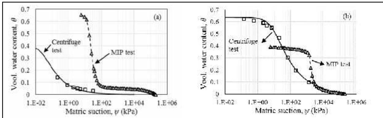
Figure 5. SWRC of single porosity soils based on centrifuge test and MIP test: a) K-7 sand, and b) Kaolin clay
