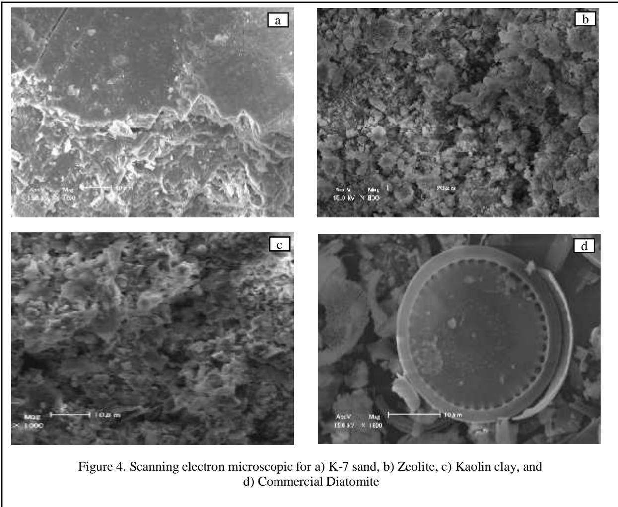
Figure 4. Scanning electron microscopic for a) K-7 sand, b) Zeolite, c) Kaolin clay, and d) Commercial Diatomite
