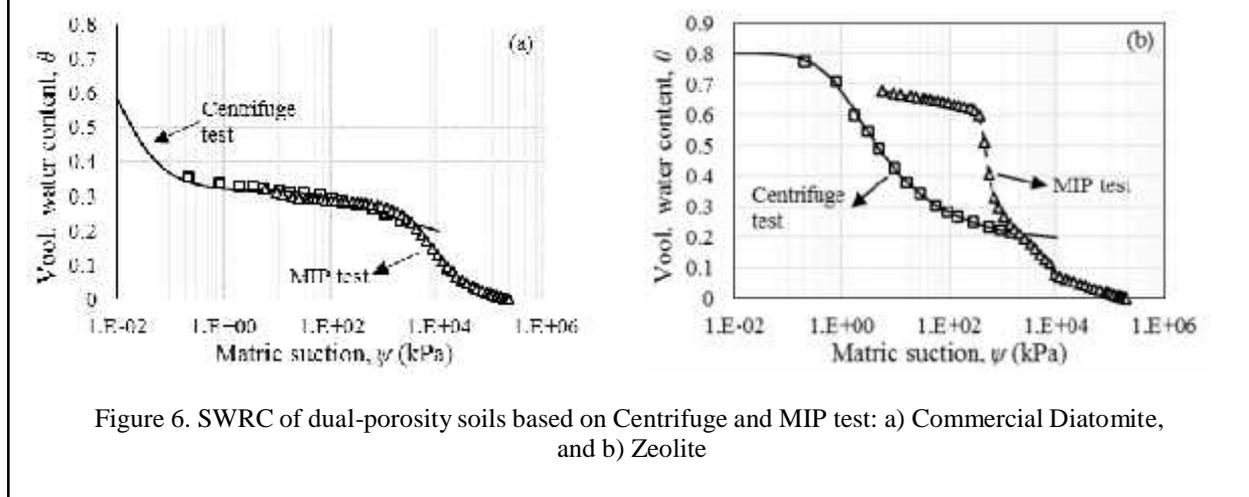
Figure 6. SWRC of dual-porosity soils based on Centrifuge and MIP test: a) Commercial Diatomite, and b) Zeolite
