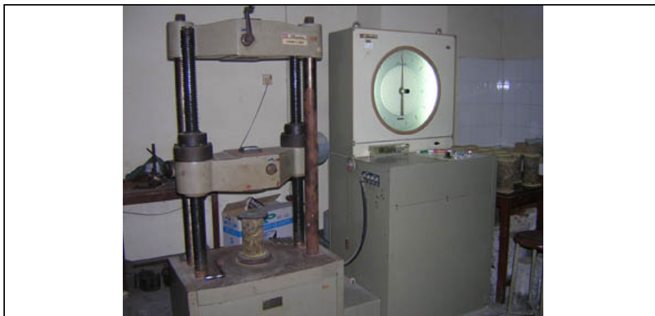
Figure 3. A cylindrical specimen went through compression strength (CS) test, using Universal Testing Machine for Load Factor (Shimadzu UMH-30). Source: Private collections
